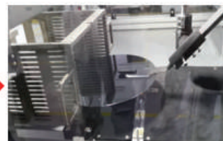
Arm Place the wafer to HAST cassette for next process
