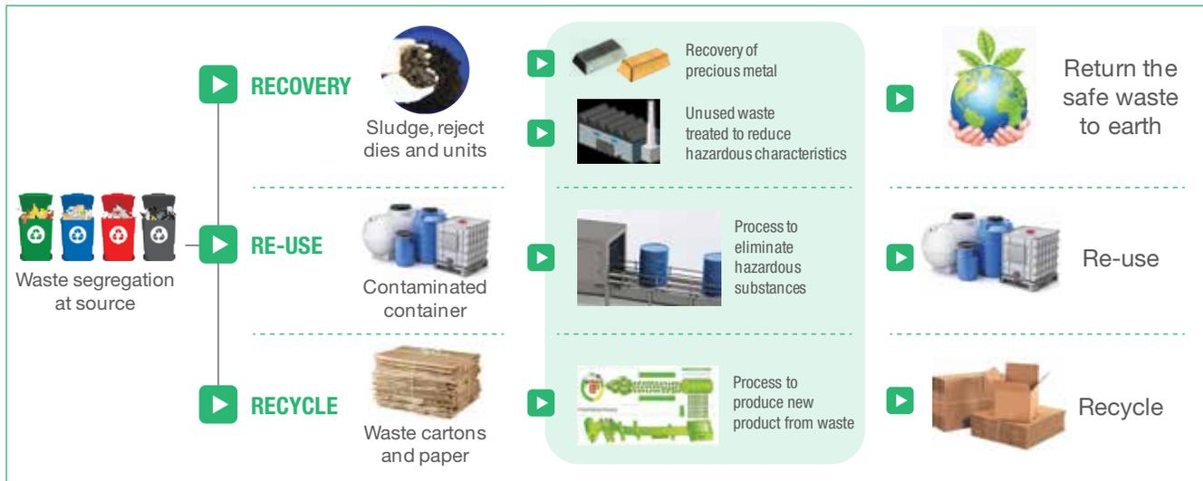
Our waste management approach also includes organic and non-organic waste chemicals. The organic waste chemicals are converted into raw materials for pesticides and water treatment solutions, while the non-organic waste chemicals are broken down to produce alcohol, thinner and solutions used by other industries. The table below presents the sample list of production waste which recovers, re-uses and recycles.
